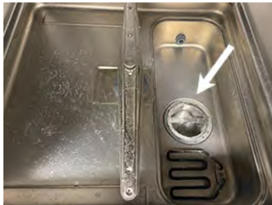
Fig. 14 Filter when option drain pump
