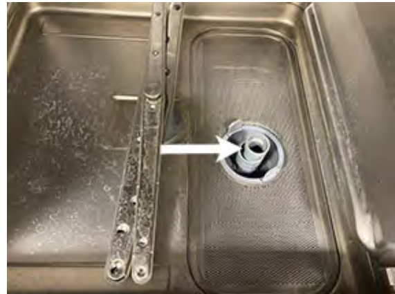
Fig. 10 Remove overflow pipe
