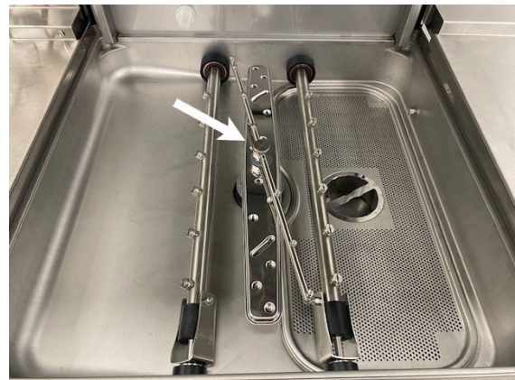
Fig. 24 Remove lower wash and rinse arms
