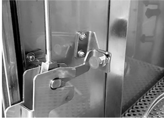
**Fig. 26 Close up – secure the arm properly**
