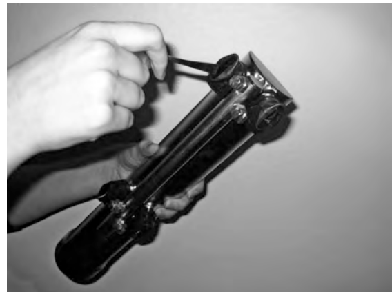
Fig. 24 Cleaning wash nozzles
