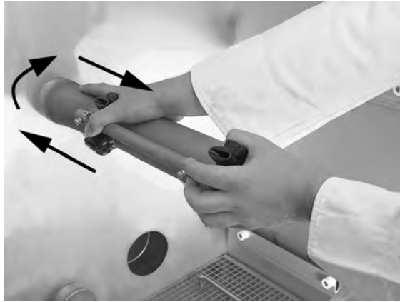
Fig. 30 Refitting of spray pipe
