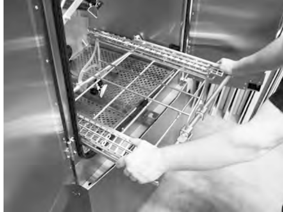
Fig. 5 Draw the insert out
