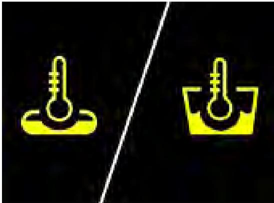
**Fig. 8 Thermostop wash or rinse tank**
